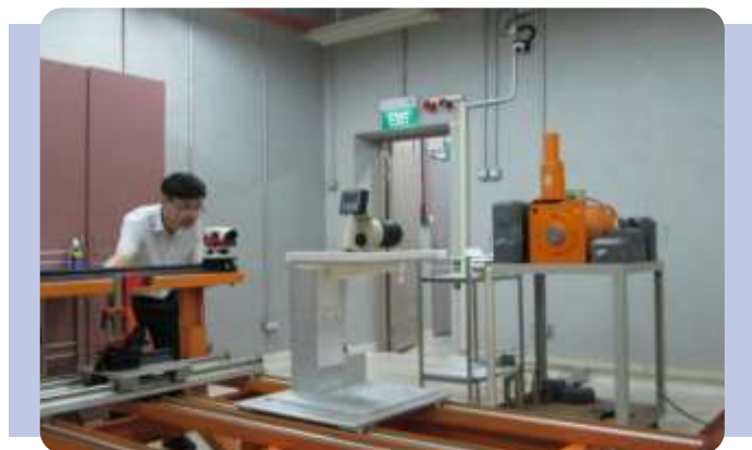
Survey meter calibration at the Secondary Standards Dosimetry Laboratory
