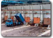
The pressure in the two waste bunkers is kept below atmospheric pressure to prevent odours from escaping. The waste in the bunker is fed by waste cranes into the six incinerators.
