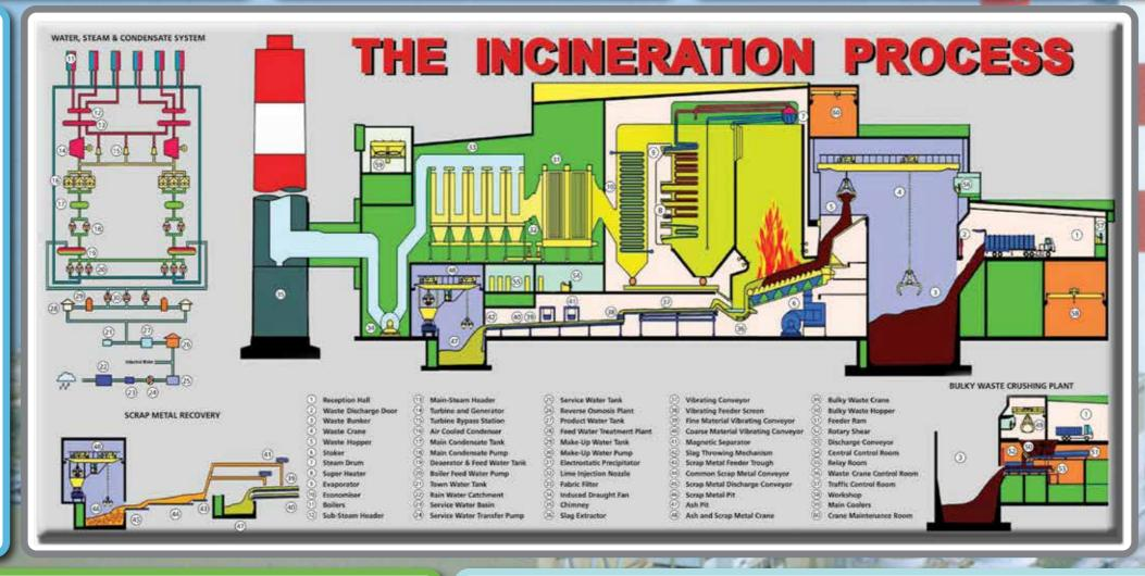
Advanced combustion control systems regulate the waste feeding and combustion rate to achieve a complete burnout of the waste.
