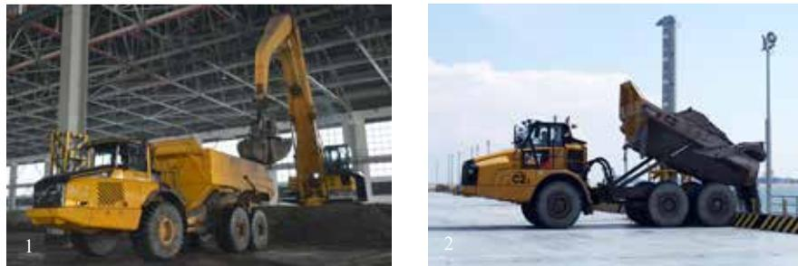
At the Semakau Transfer Building (Pic. 1), incineration ash or non-incinerable waste (NIW) being loaded into dump truck and carried to the Floating Platform or Phase I landfill cell.
