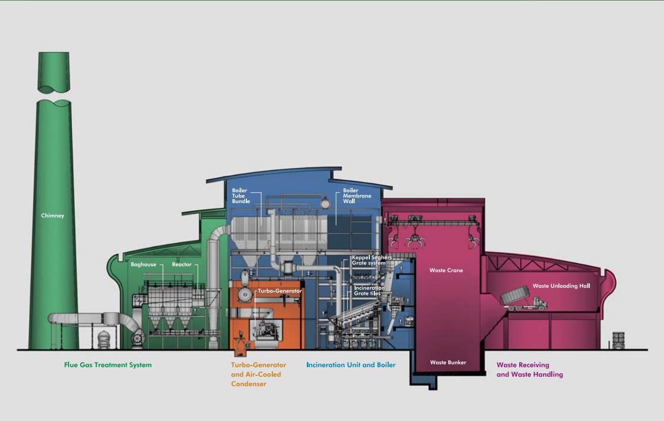
Cross section diagram of the Keppel Seghers Tuas WTE Plant:
