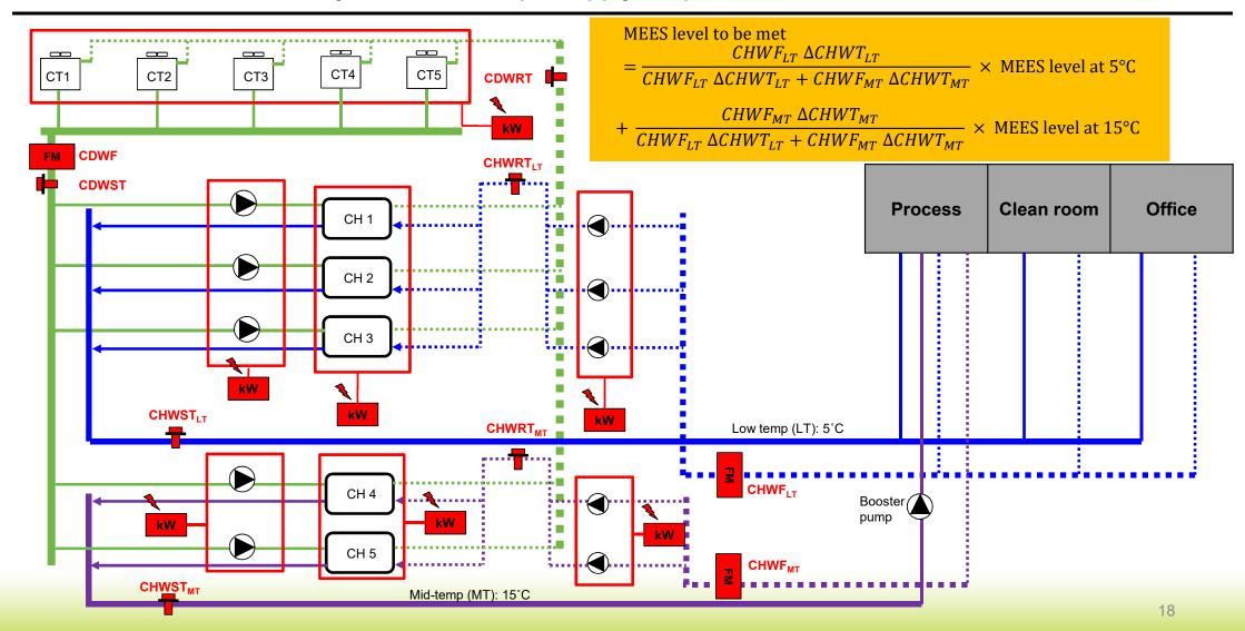
**Plant F – Chilled-Water System with Shared Cooling Towers**
