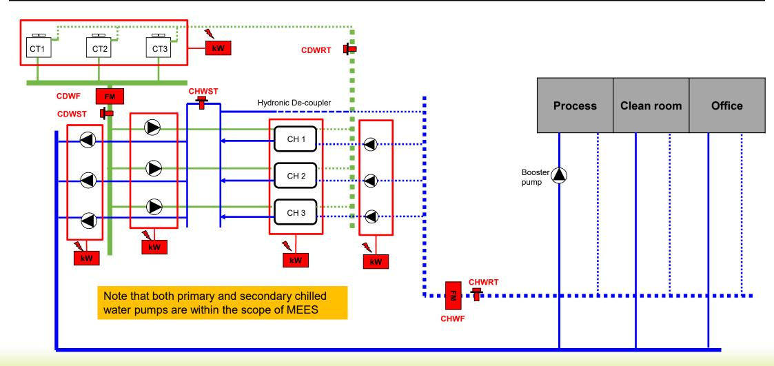
Plant D – Chilled Water System with Thermal Storage
