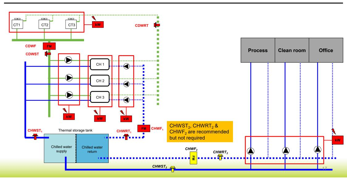
Plant E – Chilled-Water System with multiple supply temperatures
