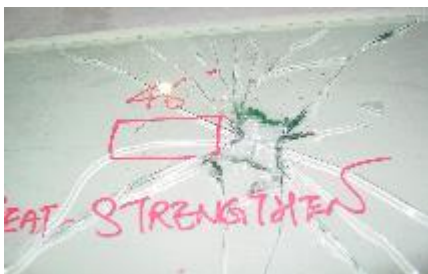
Figure 87: Heat Strengthened Glass (Courtesy: AgFacadesign & G Facadesign Pte Ltd)
