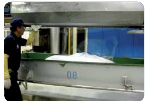
Simplified and shortened the laminating machine start-up process so that less polyethylene would drool away and be wasted
