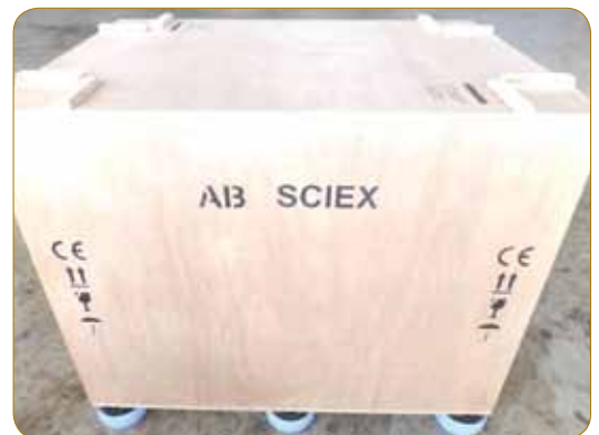
Erected re-engineered crate with skid-mates and edge guides to improve protection and shock absorption
