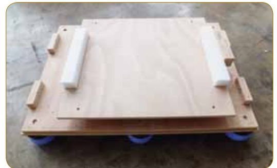
Re-engineered crate can be collapsed for easy storage and return for reuse
