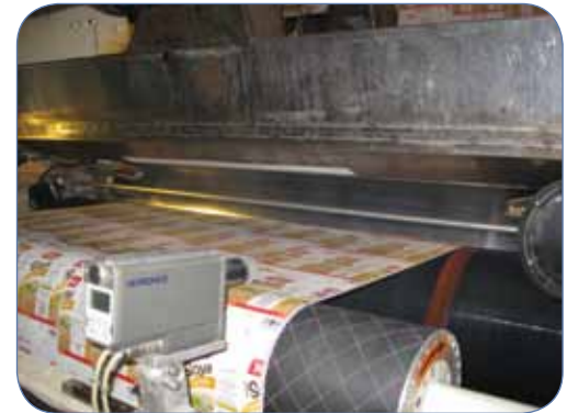
Tetra Pak implemented a standardised procedure to clean the chilled roller during temporary breaks in the lamination process
