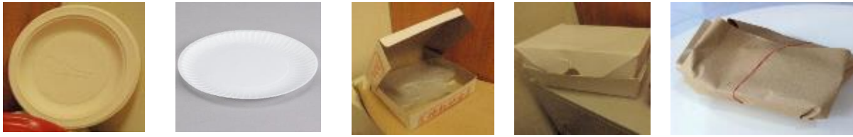
(From left to right) Corn starch plate; paper plate; paper container with inner plastic sheet, paper container with wax coating; and brown paper wrapping with plastic coating.
