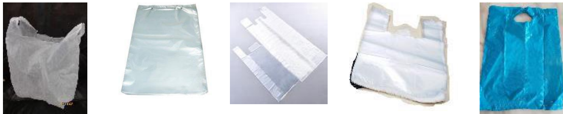
(From left to right) HDPE bag; LLDPE bag; PLA bag; corn starch bag; and oxo-degradable bag.
