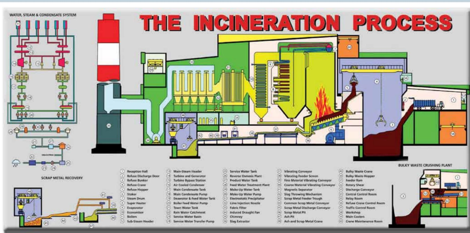
**4** Advanced combustion control systems regulate the refuse feeding and combustion rate to achieve a complete burnout of the refuse.
