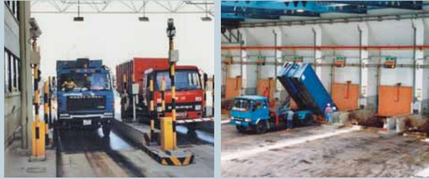
**2** The pressure in the two refuse bunkers is kept below atmospheric pressure to prevent odours from escaping. The refuse in the bunker is fed by refuse cranes into the six incinerators.
