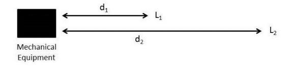
The noise level measured at distance  $d_1$  is  $L_1$  (in dBA). The <u>computed</u> noise level at distance  $d_2$  is  $L_2$  (in dBA).  $L_2 = L_1 - 20\log (d_2/d_1)$
