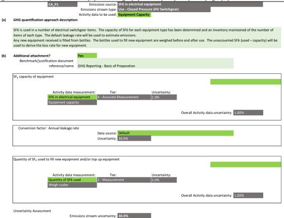
Figure 37 shows an example where a facility uses the quantity of  $SF_6$  used to top up the installed equipment to quantify the emissions from use of installed equipment. The facility selects 'Quantity used' for the 'Activity data to be used'. The quantity used to top up is determined by weighing the bottles used before and after use. The section for 'Conversion factor: Annual leakage rate' should be left blank as the quantity of  $SF_6$  topped up is measured.
