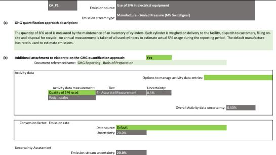
The facility using a site-specific manufacture emission rate can derive it from the quantity of  $SF_6$  used to fill the equipment compared to the capacity of the equipment:
