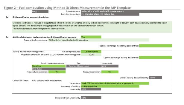
Figure 3 – Fuel combustion using Method 3: Direct Measurement, where Method 1: Calculation Approach is used for quantifying CH<sub>4</sub> and N<sub>2</sub>O emissions in the MP Template
