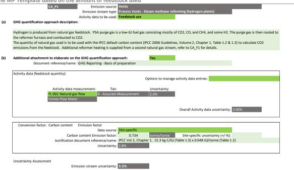
Figure 15 – Vented emissions from steam methane reforming (hydrogen plants) using Method 1: Calculation Approach in the MP Template based on amount of hydrogen produced
