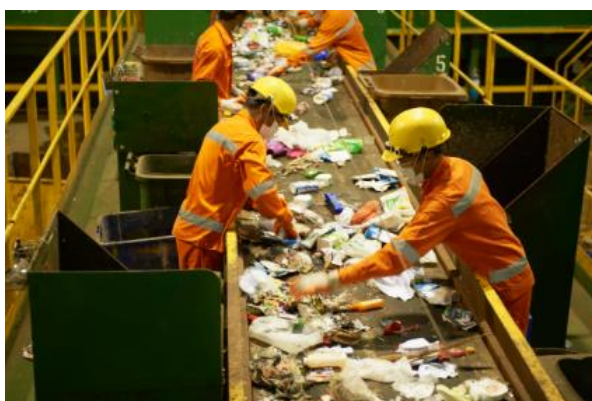
Workers sorting out recyclables at the manual sorting line at SembWaste's Materials Recovery Facility
