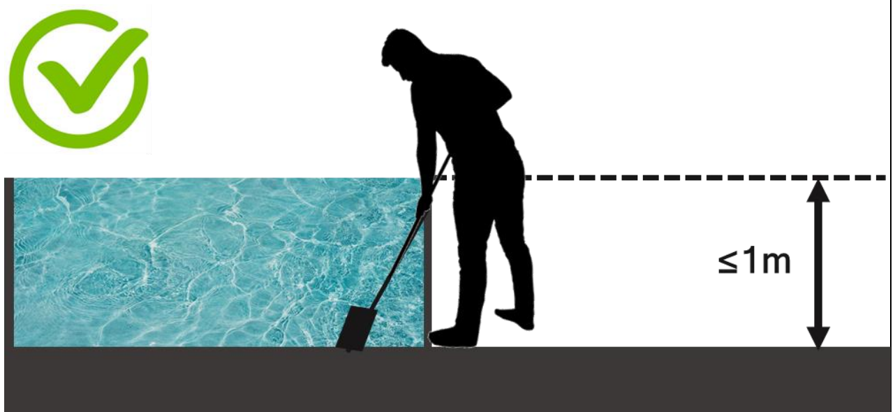
Figure 6: Maximum Allowable Barrier Height for Lowered Buffer Floor for Effective Cleaning
